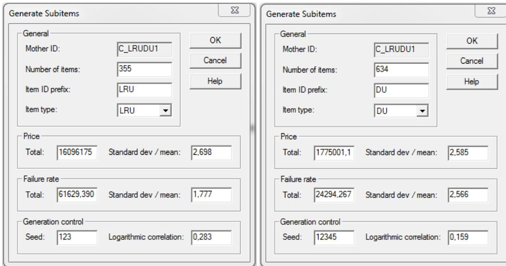
Figure 6 In OPUS10, creating the LRU:s and DU:s of a fictive system generated by high level information.
