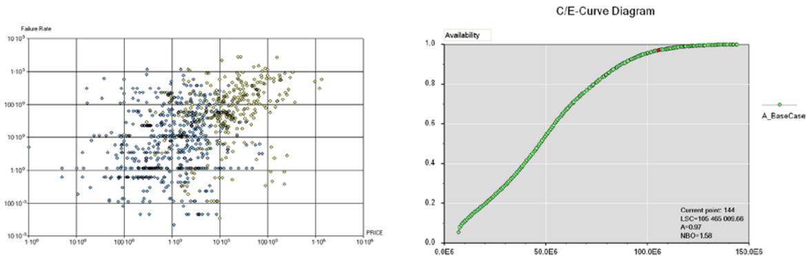
**Figure 5 A real technical system. Distribution of prices and failure rates for all items and the corresponding cost-effectiveness curve (C/E-curve) from an optimization in OPUS10.**
