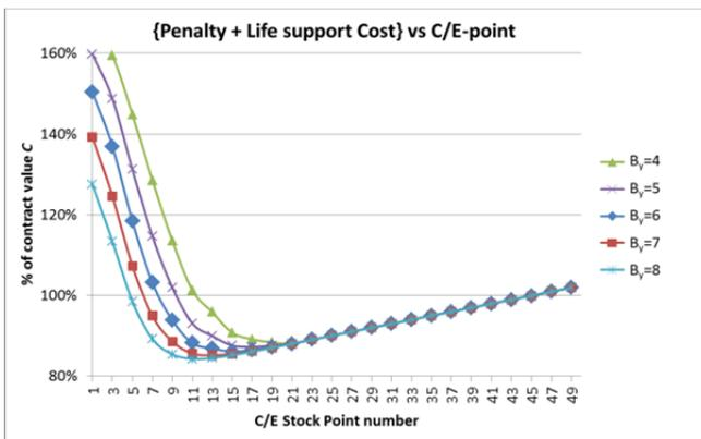
Figure 1. Supplier cost when using backorder penalty thresholds  $B_y = 4, 5, 6, 7$  and  $8$ .
